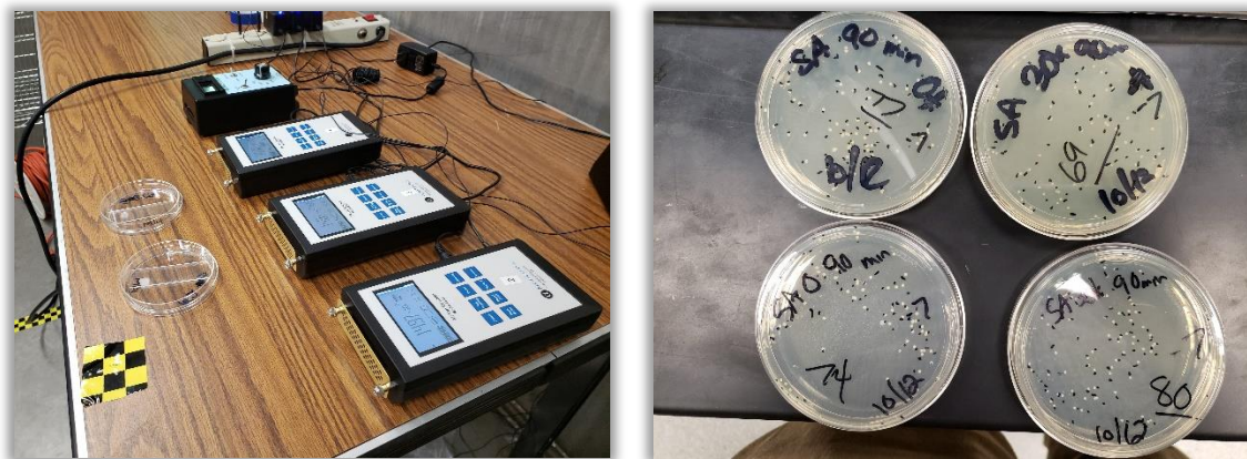
Figure 9: LEFT - Setup of Sample Slides and Ion Counters. RIGHT – Cultivated S. aureus Plates With and Without Ion Treatment
